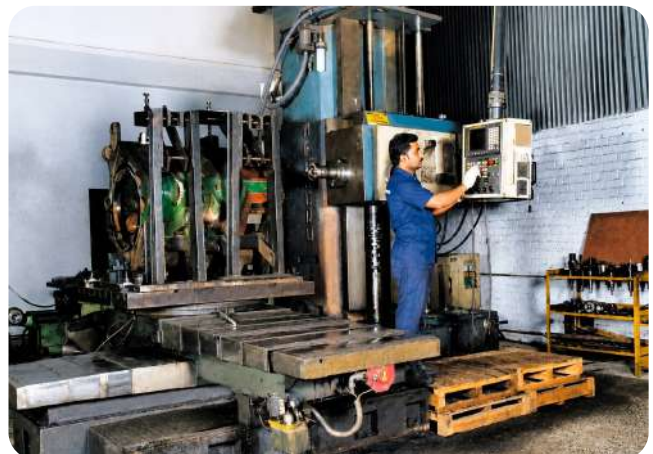
CNC BORING MACHINE
